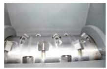
All ZERMA shredders are equipped with our E-style flat rotor. The knives are fixed in special knife holders fitted in machined pockets.
