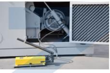
To ensure a safe operation and quick and easy access for cleaning and maintenance the GSC 500 machines cutting chamber is opened hydraulically.
