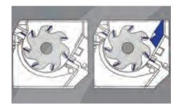
The easily removable deflector wedge acts as a third stator blade and can be used to adjust the aggressiveness of the rotor at the first cutting point.
