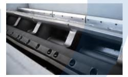
The GSH 1100 series comes standard with wide H-style rotors available with 9,11 or 13 rows of rotor blades ensuring a high quality output.
