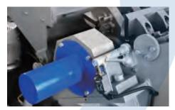
The heavy duty bearings are separated from the cutting chamber to avoid lubricants entering the cutting chamber and bearing failure due to material contamination in the bearings.
