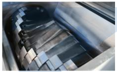
Staggered rotor blades creates an individual blade cut thus increasing the cutting torque. All of the machines in this series are therefore suitable for grinding more solid materials and thicker walled sprues.
