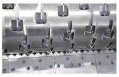
All ZERMA shredders are equipped with a large diameter flat rotor. The knives are fixed in special knife holders fitted in machined pockets. Optional weld on hard facing is available for abrasive applications.
