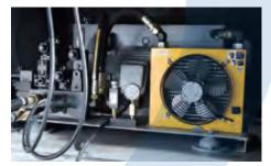
The ZXS shredders feature a high powered twin speed hydraulic system. This system ensures maximum pressure when feeding material into the rotor and high speeds on the backstroke.
