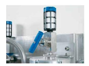
All stainless steel parts are made of non corrosive 316 stainless steel
