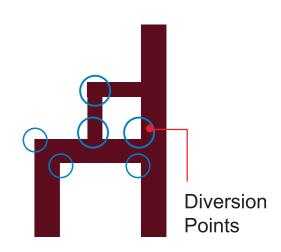
If the molding parts is flat shape (as bottom sample, it is a plate.), wooden pattern or marble effects will not occur as no diversion point inside the mold.
