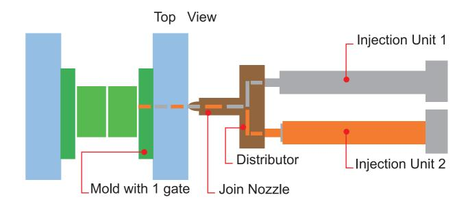
This is the system produced parts as chair or other plastic products,2 (or 3 or 4) different colors of plastic material from separate barrel mixed in a distributor, the mixed material go into the Joint Nozzle, and the mixed material from Joint Nozzle into the mold from one gate. (The mold with only 1 gate / Distributor is a parts of machine.)
