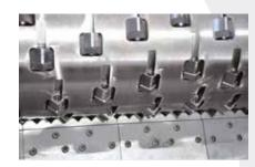
All ZERMA shredders are equipped with a large diameter flat rotor. The knives are fixed in special knife holders fitted in machined pockets. Optional weld on hard facing is available for abrasive applications.
