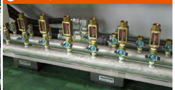
9 Mold cooling water closed circuit on bed
