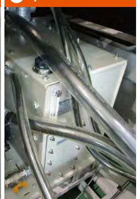
9 Mold cooling water closed circuit on bed
